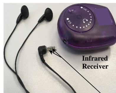
Earphones with 3.5 mm diameter plug Insulating rings
